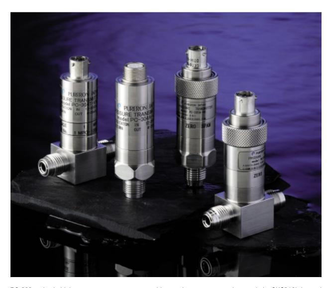
PC-300 series is high accuracy pressure sensor with superior temperature characteristic. SUS316L is used for gas (fluid) contacting area for superior corrosion resistance. Selectable output either 4 to 20mA, 0 to 5V or 0 to 10V enables easy connection with various digital panel meters and programmable controllers.
