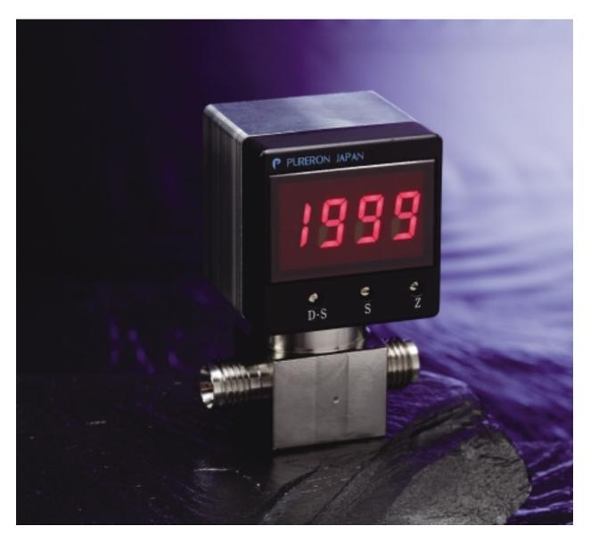
PCD-905 series is high accuracy pressure sensor with indicator having superior temperature characteristic. SUS316L is used for gas (fluid) contacting area for superior corrosion resistance. Output is 0 to 5V to be connected with various digital panel meters and programmable controllers.
