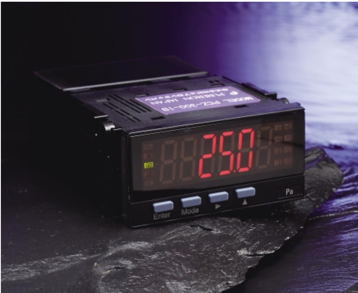
PCZ-300 series is high performance micro differential pressure gauge measurable from minimal pressure at 25Pa. By adopting flow sensor instead of diaphragm for pressure-sensing part, superior repeat accuracy is achieved without affected by mounting orientation. And there is no concern over zero drift.
